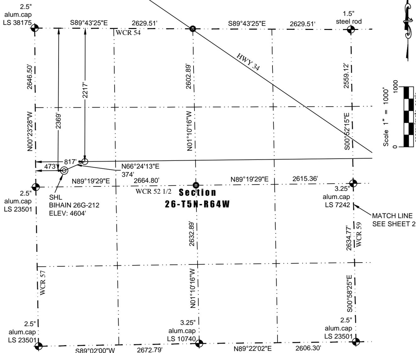
In accordance with a request from Barney Hammond of PDC Energy, Inc., Washburn Land Surveying, LLC has determined the location of the **BIHAIN 26G-212** well site to be SHL: 2369' FNL and 473' FWL, (BHL: 2200' FNL and 500' FEL), as measured at ninety (90) degrees from the section lines of Sections 26 and 25, Township 5 North, Range 64 West of the 6th Principal Meridian, Weld County Colorado.
