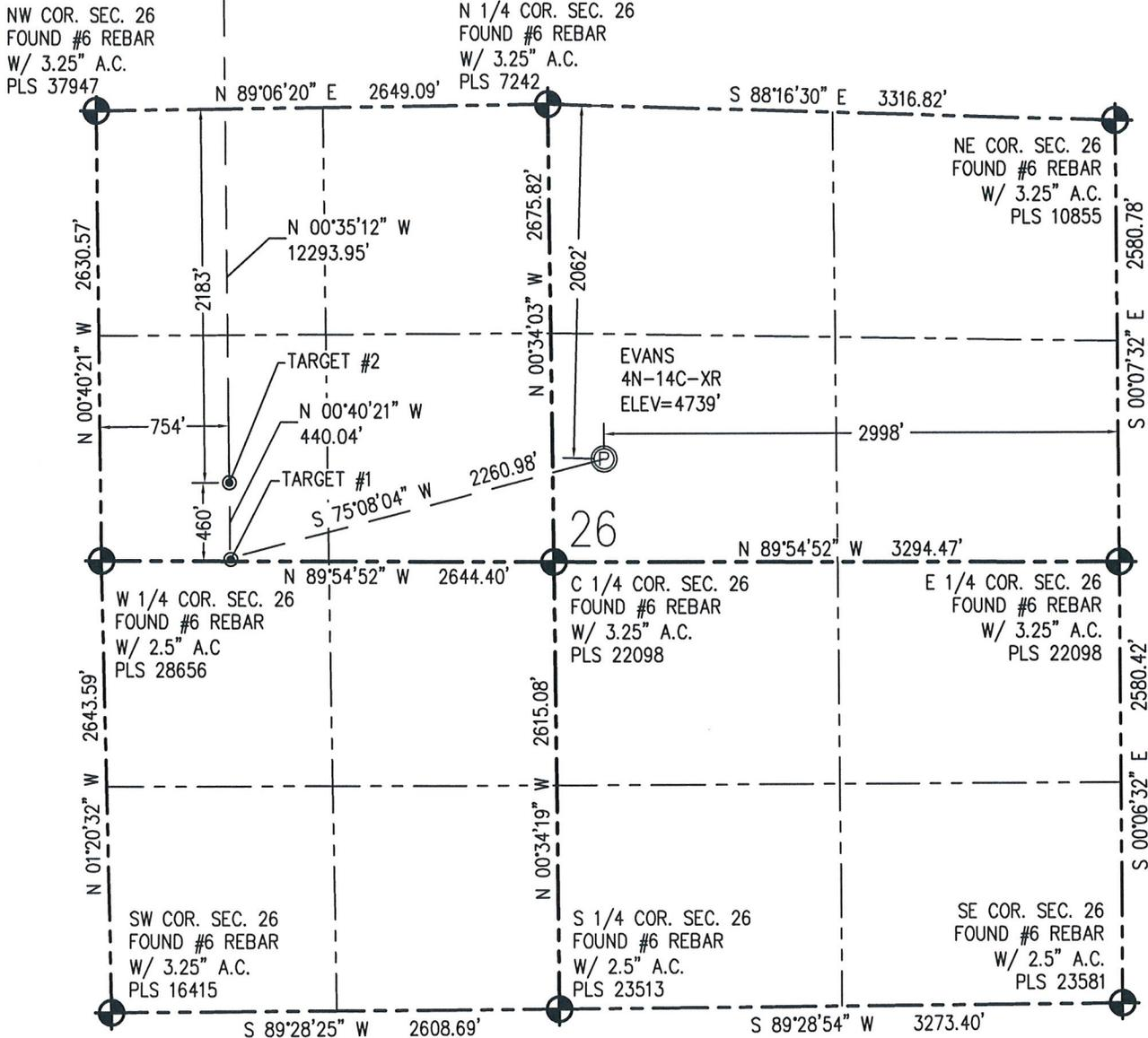
**N** IN ACCORDANCE WITH A REQUEST FROM CRAIG RASMUSON - SYNERGY RESOURCES, BASELINE ENGINEERING CORP. HAS DETERMINED THE LOCATION OF THE EVANS 4N-14C-XR TO BE 2062' FNL AND 2998' FEL, AS MEASURED AT NINETY (90) DEGREES FROM THE SECTION LINE OF SECTION 26, TOWNSHIP 5 NORTH, RANGE 66 WEST AND THE BOTTOM HOLE LOCATION TO BE 460' FNL AND 754' FWL OF SECTION 14, TOWNSHIP 5 NORTH, RANGE 66 WEST, 6TH PRINCIPAL MERIDIAN, WELD COUNTY, COLORADO.
