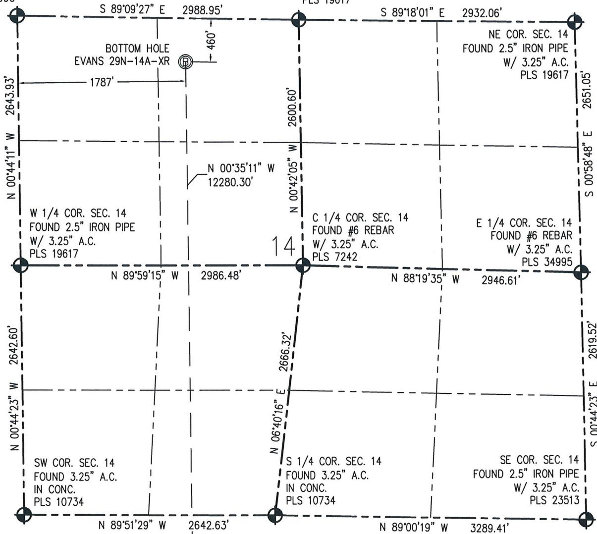
**N** IN ACCORDANCE WITH A REQUEST FROM CRAIG RASMUSON - SYNERGY RESOURCES, BASELINE ENGINEERING CORP. HAS DETERMINED THE LOCATION OF THE EVANS 29N-14A-XR TO BE 1942' FNL AND 2999' FEL, AS MEASURED AT NINETY (90) DEGREES FROM THE SECTION LINE OF SECTION 26, TOWNSHIP 5 NORTH, RANGE 66 WEST AND THE BOTTOM HOLE LOCATION TO BE 460' FNL AND 1787' FWL OF SECTION 14, TOWNSHIP 5 NORTH, RANGE 66 WEST, 6TH PRINCIPAL MERIDIAN, WELD COUNTY, COLORADO.
