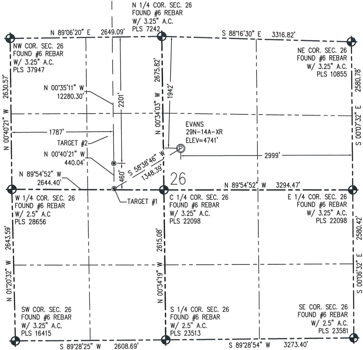
**N** IN ACCORDANCE WITH A REQUEST FROM CRAIG RASMUSON - SYNERGY RESOURCES, BASELINE ENGINEERING CORP. HAS DETERMINED THE LOCATION OF THE EVANS 29N-14A-XR TO BE 1942' FNL AND 2999' FEL, AS MEASURED AT NINETY (90) DEGREES FROM THE SECTION LINE OF SECTION 26, TOWNSHIP 5 NORTH, RANGE 66 WEST AND THE BOTTOM HOLE LOCATION TO BE 460' FNL AND 1787' FWL OF SECTION 14, TOWNSHIP 5 NORTH, RANGE 66 WEST, 6TH PRINCIPAL MERIDIAN, WELD COUNTY, COLORADO.
