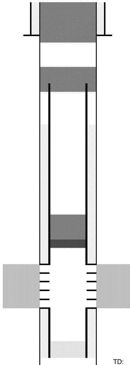
Cut surface casing off 6'-8' below surface.
