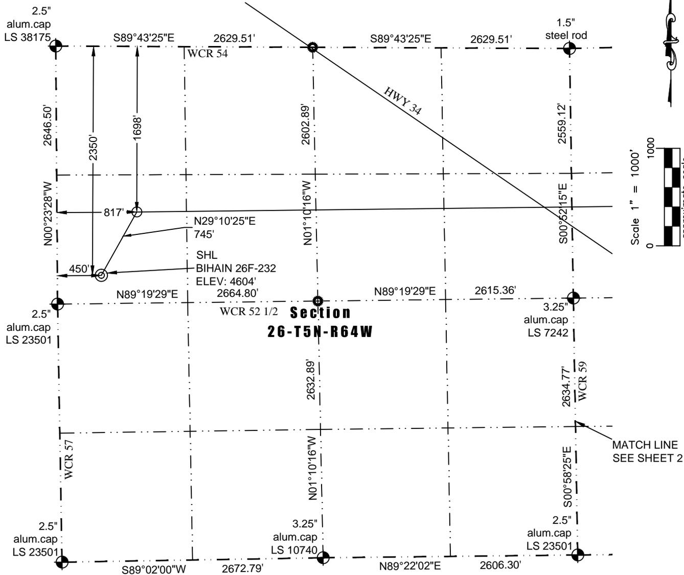
In accordance with a request from Barney Hammond of PDC Energy, Inc., Washburn Land Surveying, LLC has determined the location of the **BIHAIN 26F-232** well site to be SHL: 2350' FNL and 450' FWL, (BHL: 1680' FNL and 500' FEL), as measured at ninety (90) degrees from the section lines of Sections 26 and 25, Township 5 North, Range 64 West of the 6th Principal Meridian, Weld County Colorado.
