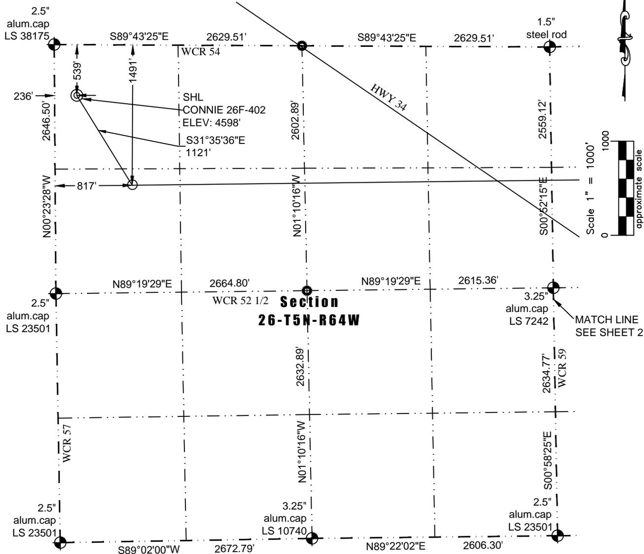
In accordance with a request from Barney Hammond of PDC Energy, Inc., Washburn Land Surveying, LLC has determined the location of the **CONNIE 26F-402** well site to be SHL: 539' FNL and 236' FWL, (BHL: 1470' FNL and 500' FEL), as measured at ninety (90) degrees from the section lines of Sections 26 and 25, Township 5 North, Range 64 West of the 6th Principal Meridian, Weld County Colorado.
