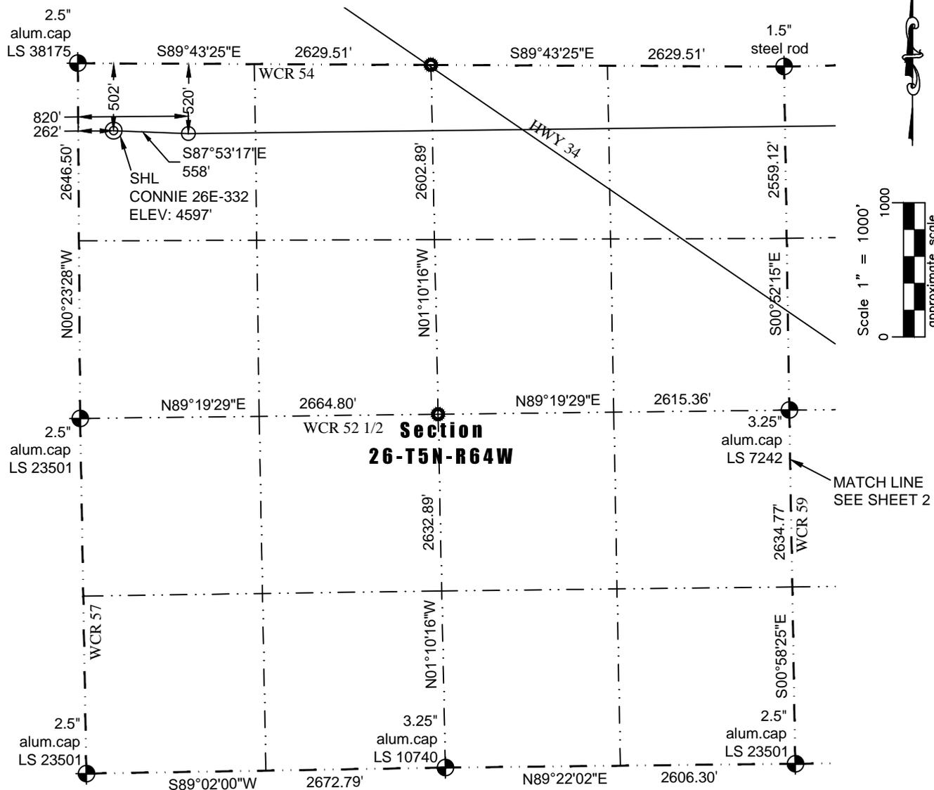
In accordance with a request from Barney Hammond of PDC Energy, Inc., Washburn Land Surveying, LLC has determined the location of the **CONNIE 26E-332** well site to be SHL: 502' FNL and 262' FWL, (BHL: 500' FNL and 500' FEL), as measured at ninety (90) degrees from the section lines of Sections 26 and 25, Township 5 North, Range 64 West of the 6th Principal Meridian, Weld County Colorado.
