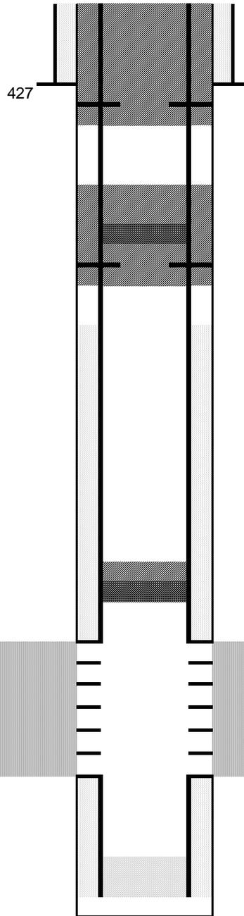
Cut surface casing off 6'-8' below surface.
