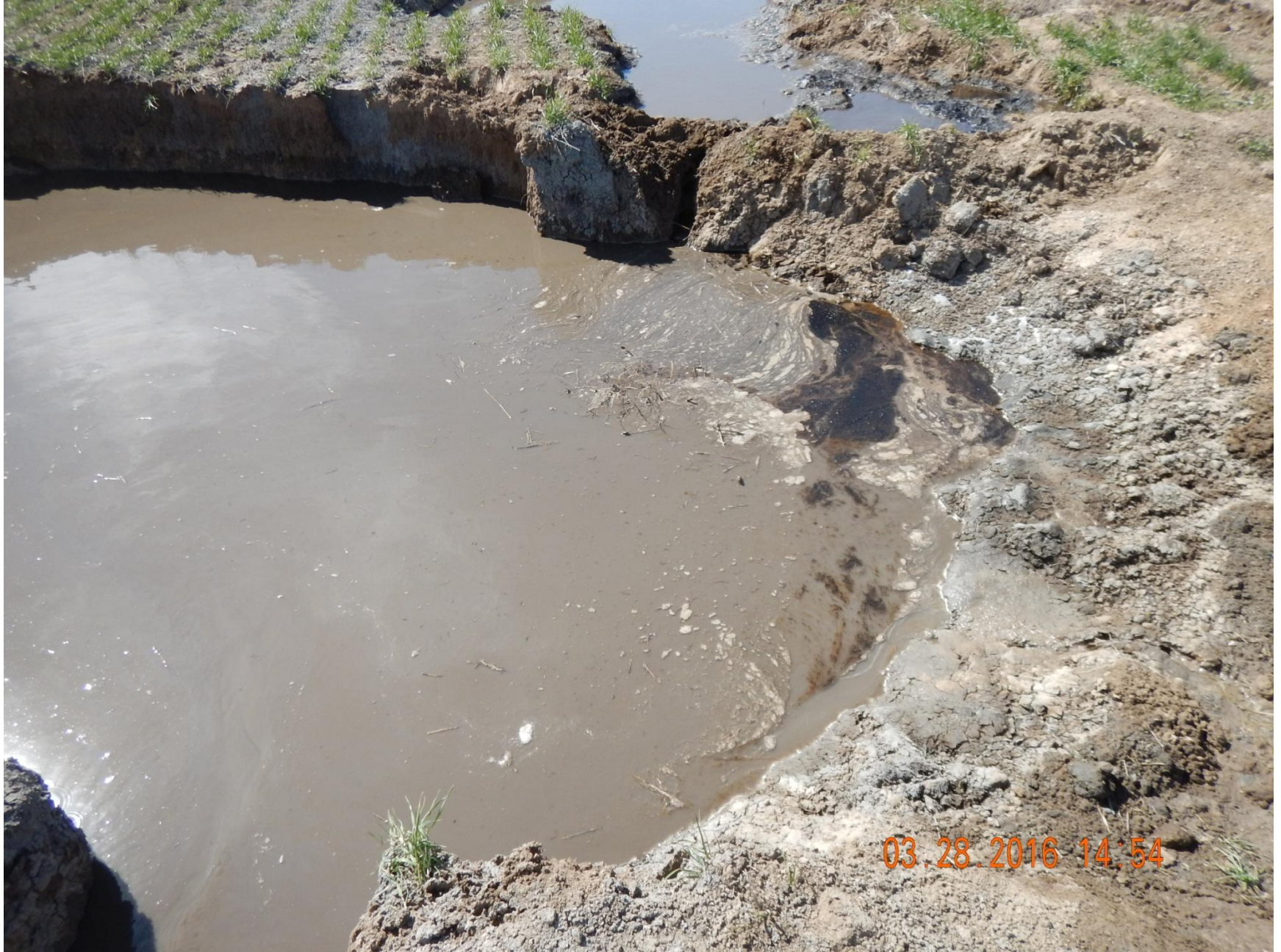
Figure 1: Photo taken from the pit on location. Photo shows oily substance on water. Likely hydraulic fluids from equipment.
