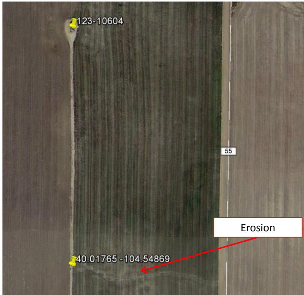
Photo 3. Google Earth aerial photo taken 10/9/2015. Erosion and transport of sediment initiates on the lease road and travels east through cropland.
