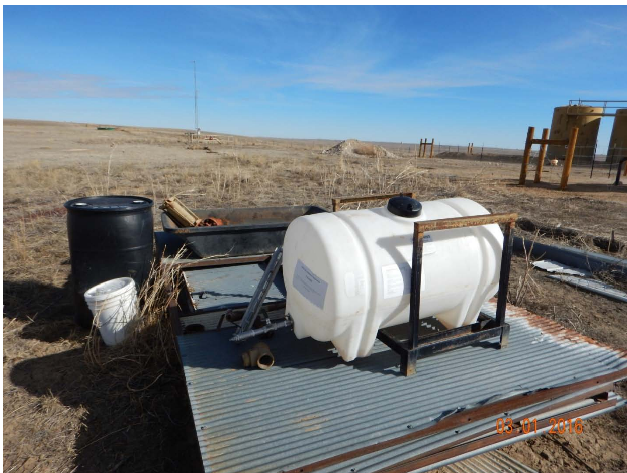
Figure 4 - Chemicals stored on-location (black 55 gallon drum and white 5 gallon bucket contained unknown material) lacking secondary containment
