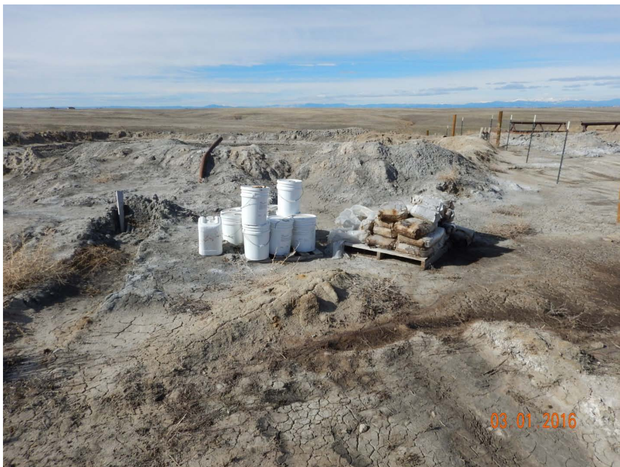
Figure 6 - Unused dry chemicals at northeast corner of fenced-in pit area. Note stained soil in foreground leads to puddle just north of fenced-in pit area.
