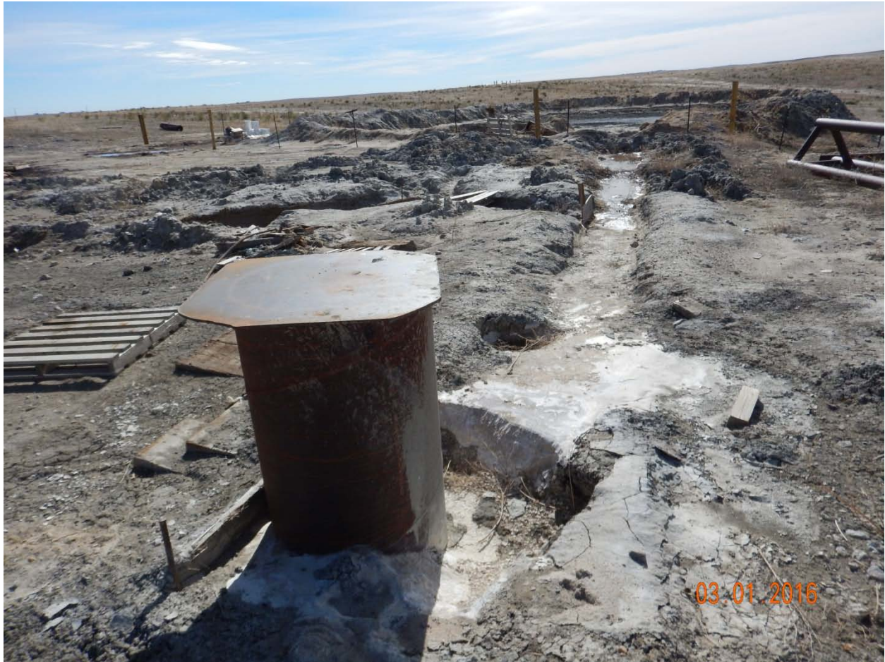
Figure 12 - Abandoned wellhead with ~2'x50' ditch leading to pit.
