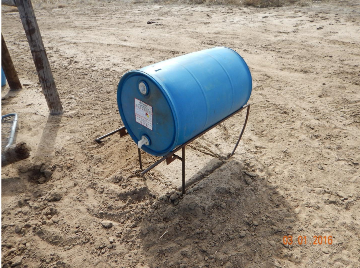
Figure 14 - 55-gallon drum outside of separator shed lacking secondary containment.
