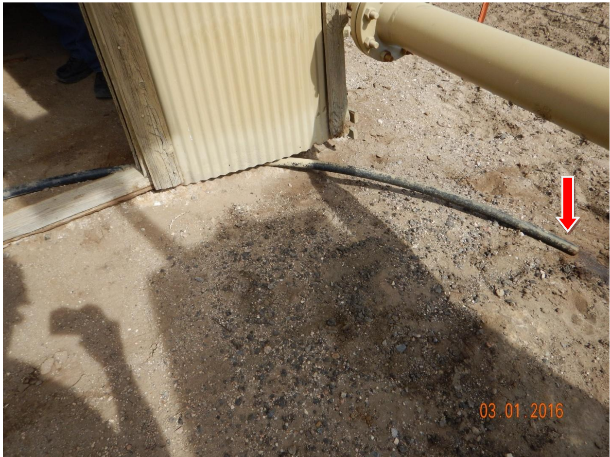
Figure 16 - Oil-stained soil at southeast corner of separator shed, note line being used to drain E&P waste from inside of shed.
