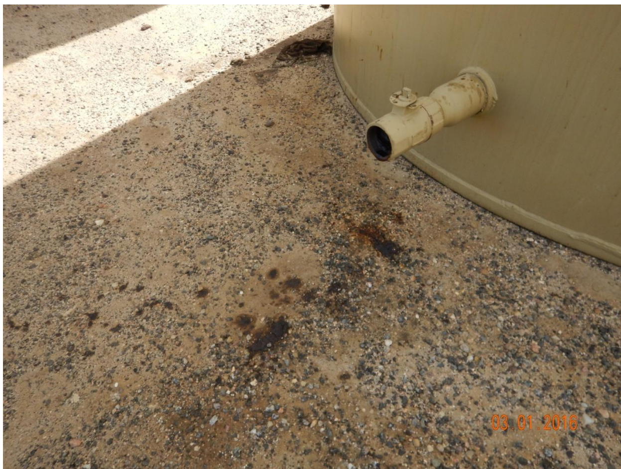
Figure 10 - Oil-stained soil north of production water tank.
