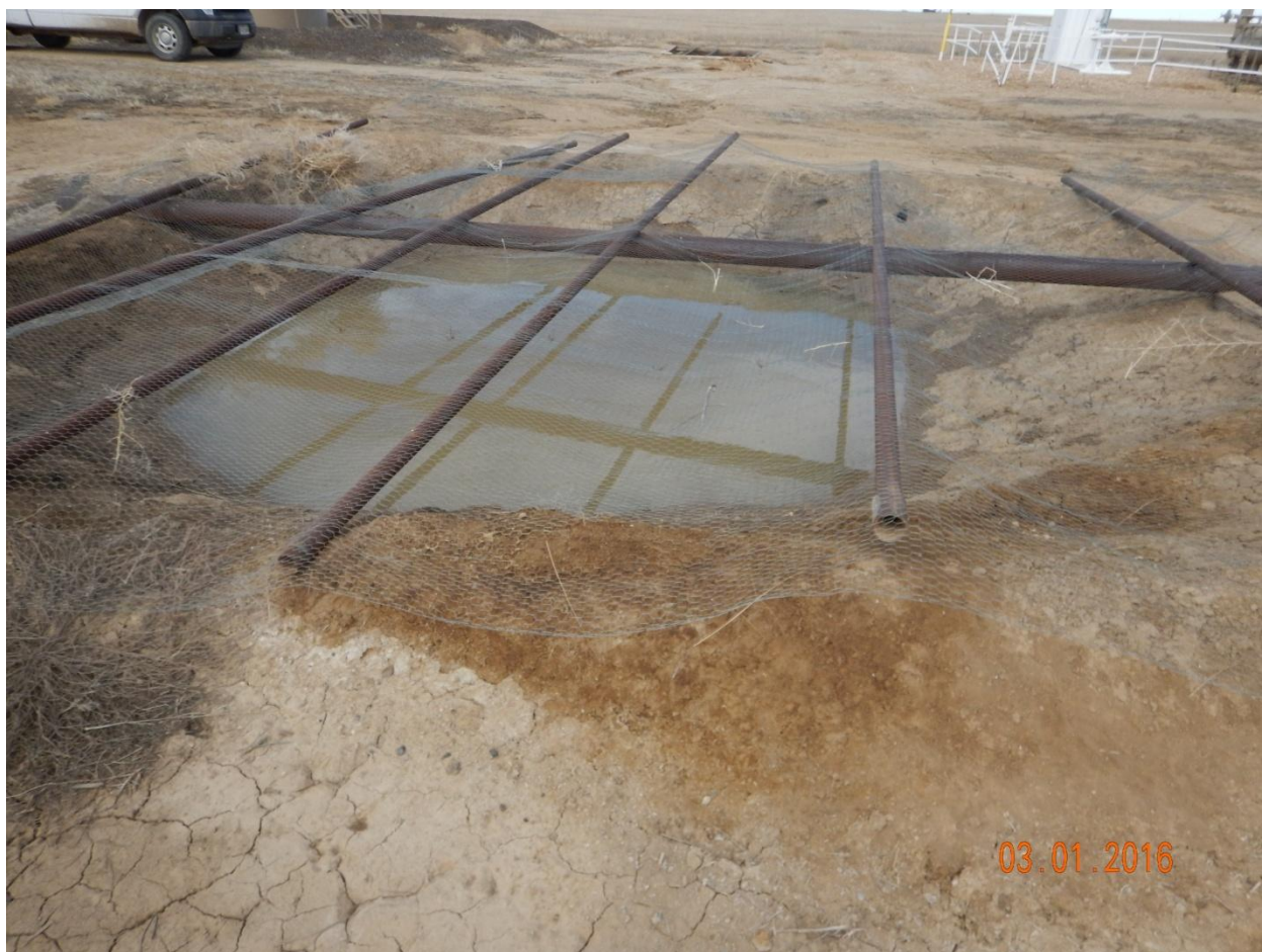
Figure 5 - Oil-stained soil at southeast corner of produced water pit. Note burrows in NE corner of pit.
