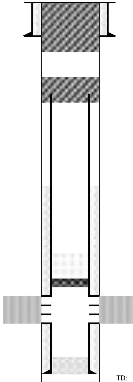
Cut surface casing off 6'-8' below surface.
