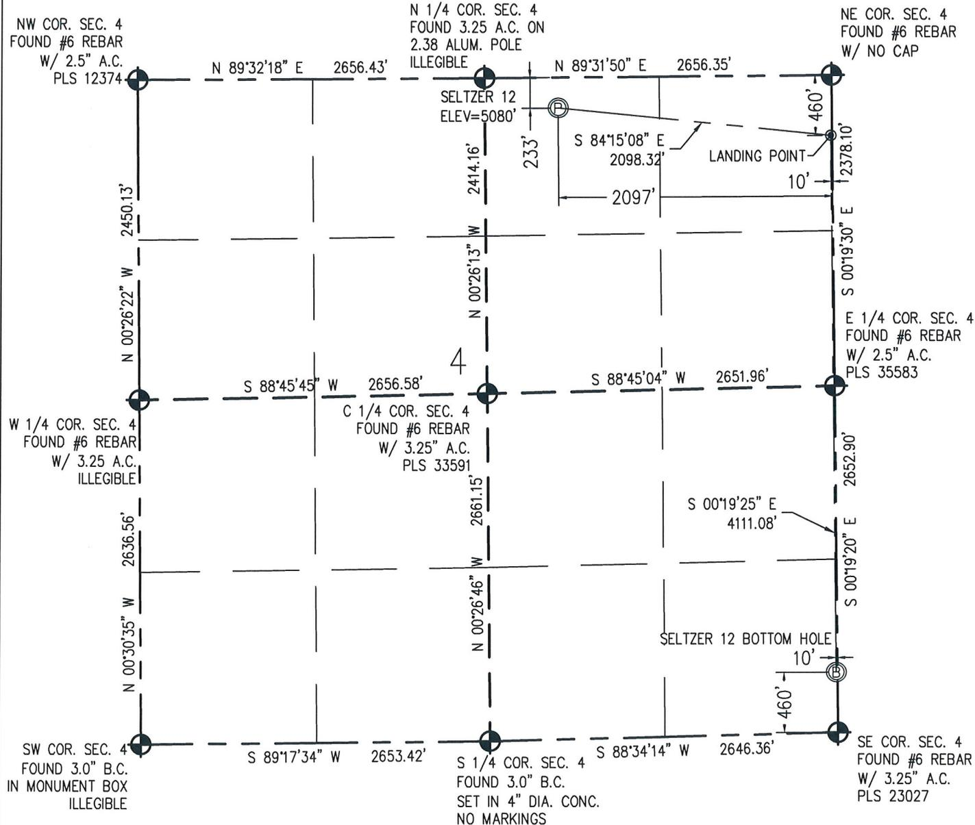
**N** IN ACCORDANCE WITH A REQUEST FROM JOSEPH SILIPO - EXTRACTION, BASELINE ENGINEERING CORP. HAS DETERMINED THE LOCATION OF THE SELTZER 12 TO BE 233' FNL AND 2097' FEL, AS MEASURED AT NINETY (90) DEGREES FROM THE SECTION LINE OF SECTION 4, TOWNSHIP 1 SOUTH, RANGE 67 WEST AND THE BOTTOM HOLE LOCATION TO BE 460' FSL AND 10' FEL OF SECTION 4, TOWNSHIP 1 SOUTH, RANGE 67 WEST, 6TH PRINCIPAL MERIDIAN, ADAMS COUNTY, COLORADO.
