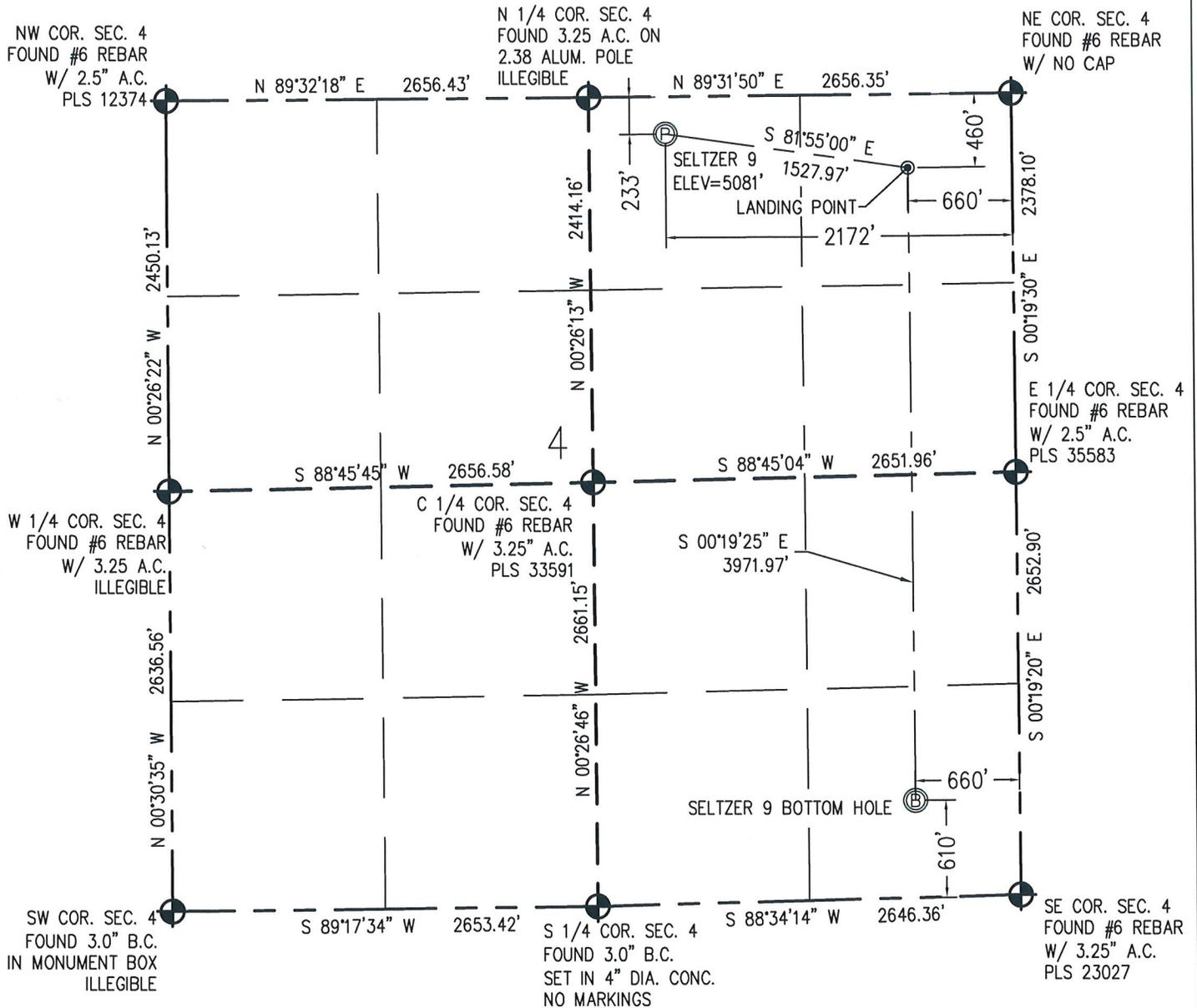
**N** IN ACCORDANCE WITH A REQUEST FROM JOSEPH SILIPO - EXTRACTION, BASELINE ENGINEERING CORP. HAS DETERMINED THE LOCATION OF THE SELTZER 9 TO BE 233' FNL AND 2172' FEL, AS MEASURED AT NINETY (90) DEGREES FROM THE SECTION LINE OF SECTION 4, TOWNSHIP 1 SOUTH, RANGE 67 WEST AND THE BOTTOM HOLE LOCATION TO BE 610' FSL AND 660' FEL OF SECTION 4, TOWNSHIP 1 SOUTH, RANGE 67 WEST, 6TH PRINCIPAL MERIDIAN, ADAMS COUNTY, COLORADO.
