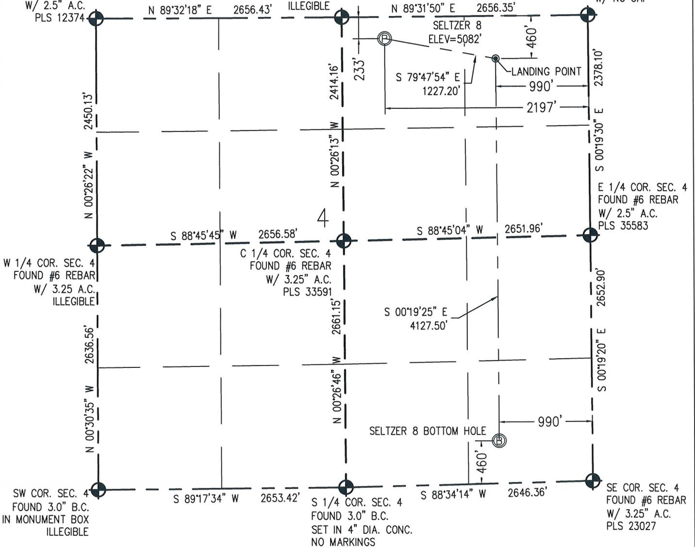
**N** IN ACCORDANCE WITH A REQUEST FROM JOSEPH SILIPO - EXTRACTION, BASELINE ENGINEERING CORP. HAS DETERMINED THE LOCATION OF THE SELTZER 8 TO BE 233' FNL AND 2197' FEL, AS MEASURED AT NINETY (90) DEGREES FROM THE SECTION LINE OF SECTION 4, TOWNSHIP 1 SOUTH, RANGE 67 WEST AND THE BOTTOM HOLE LOCATION TO BE 460' FSL AND 990' FEL OF SECTION 4, TOWNSHIP 1 SOUTH, RANGE 67 WEST, 6TH PRINCIPAL MERIDIAN, ADAMS COUNTY, COLORADO.
