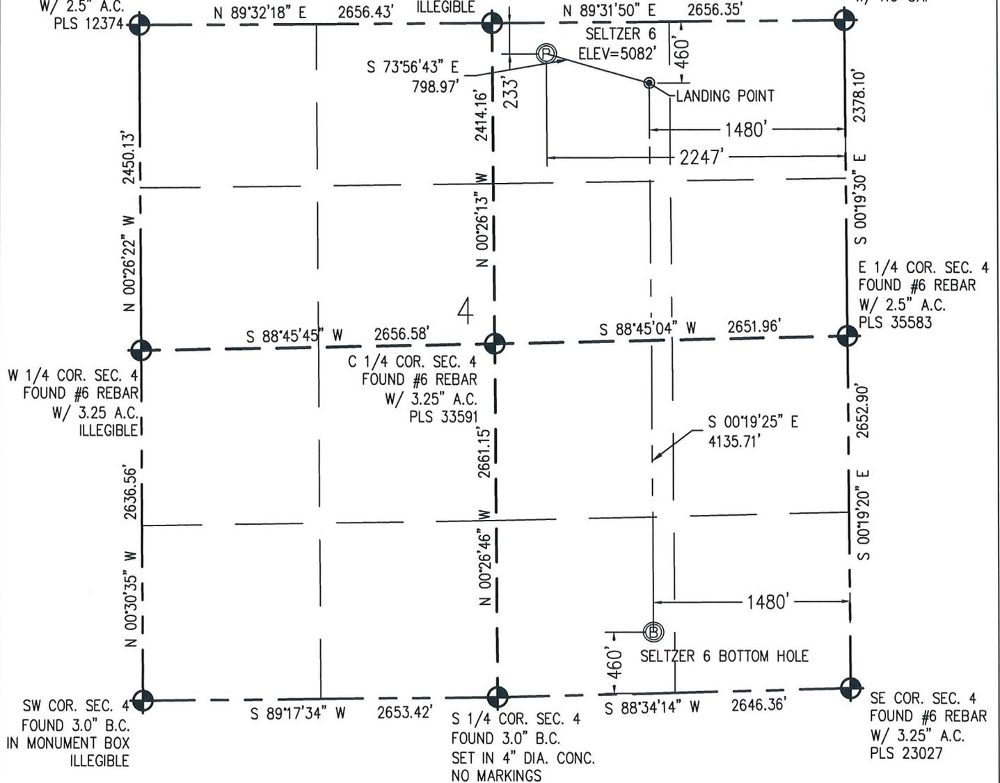
**N** IN ACCORDANCE WITH A REQUEST FROM JOSEPH SILIPO - EXTRACTION, BASELINE ENGINEERING CORP. HAS DETERMINED THE LOCATION OF THE SELTZER 6 TO BE 233' FNL AND 2247' FEL, AS MEASURED AT NINETY (90) DEGREES FROM THE SECTION LINE OF SECTION 4, TOWNSHIP 1 SOUTH, RANGE 67 WEST AND THE BOTTOM HOLE LOCATION TO BE 460' FSL AND 1480' FEL OF SECTION 4, TOWNSHIP 1 SOUTH, RANGE 67 WEST, 6TH PRINCIPAL MERIDIAN, ADAMS COUNTY, COLORADO.
