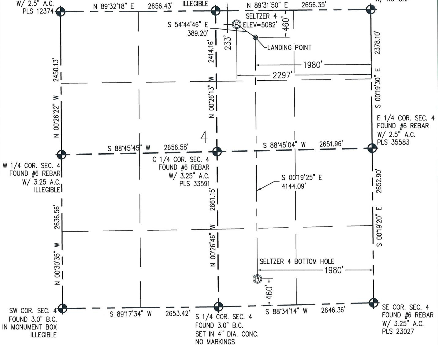
IN ACCORDANCE WITH A REQUEST FROM JOSEPH SILIPO - EXTRACTION, BASELINE ENGINEERING CORP. HAS DETERMINED THE LOCATION OF THE SELTZER 4 TO BE 233' FNL AND 2297' FEL, AS MEASURED AT NINETY (90) DEGREES FROM THE SECTION LINE OF SECTION 4, TOWNSHIP 1 SOUTH, RANGE 67 WEST AND THE BOTTOM HOLE LOCATION TO BE 460' FSL AND 1980' FEL OF SECTION 4, TOWNSHIP 1 SOUTH, RANGE 67 WEST, 6TH PRINCIPAL MERIDIAN, ADAMS COUNTY, COLORADO.
