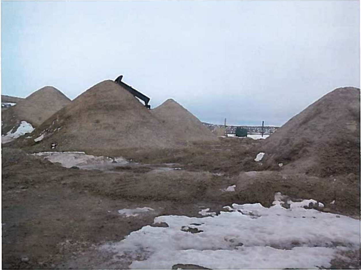
Picture taken looking South-east: E&P waste containment observed to be inadequate, E&P waste should be maintained per Rule 907.
