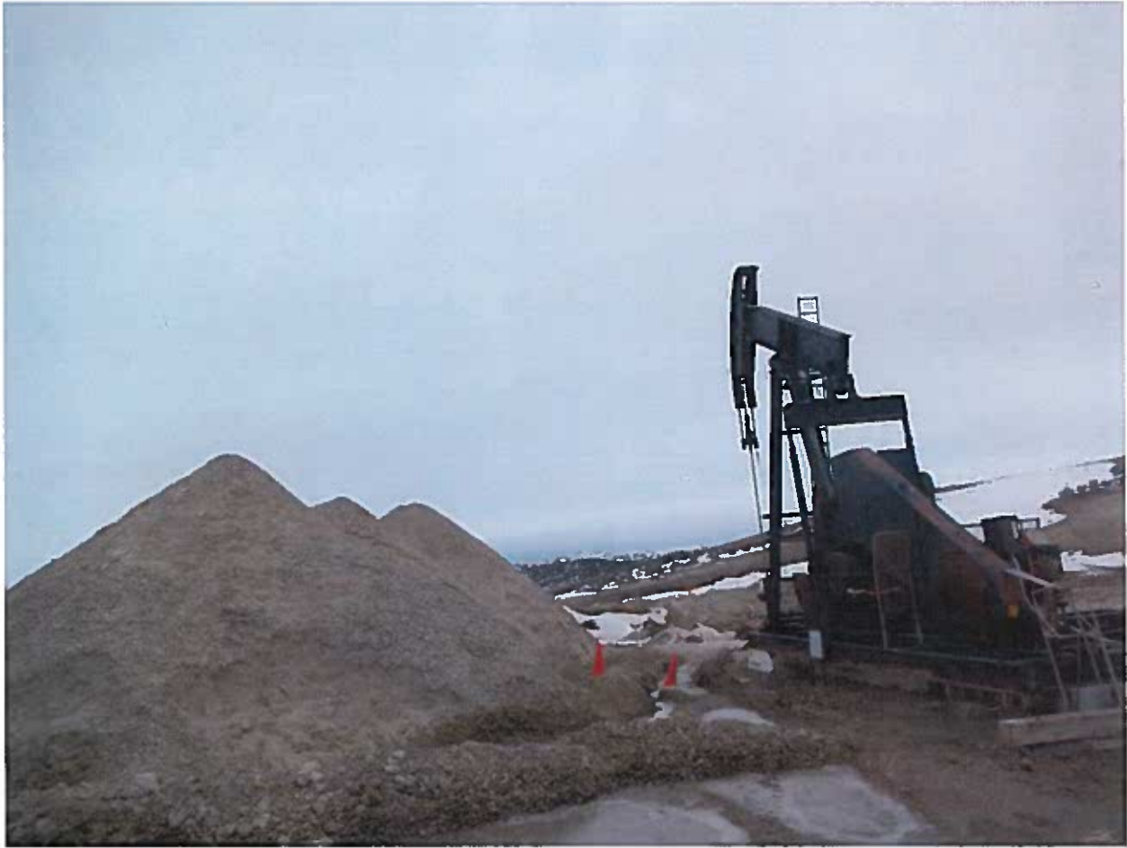
Picture taken looking North: E&P waste containment observed to be inadequate, E&P waste should be maintained per Rule 907. Waste piles appear to be in the same location as they came off the soil treater.
