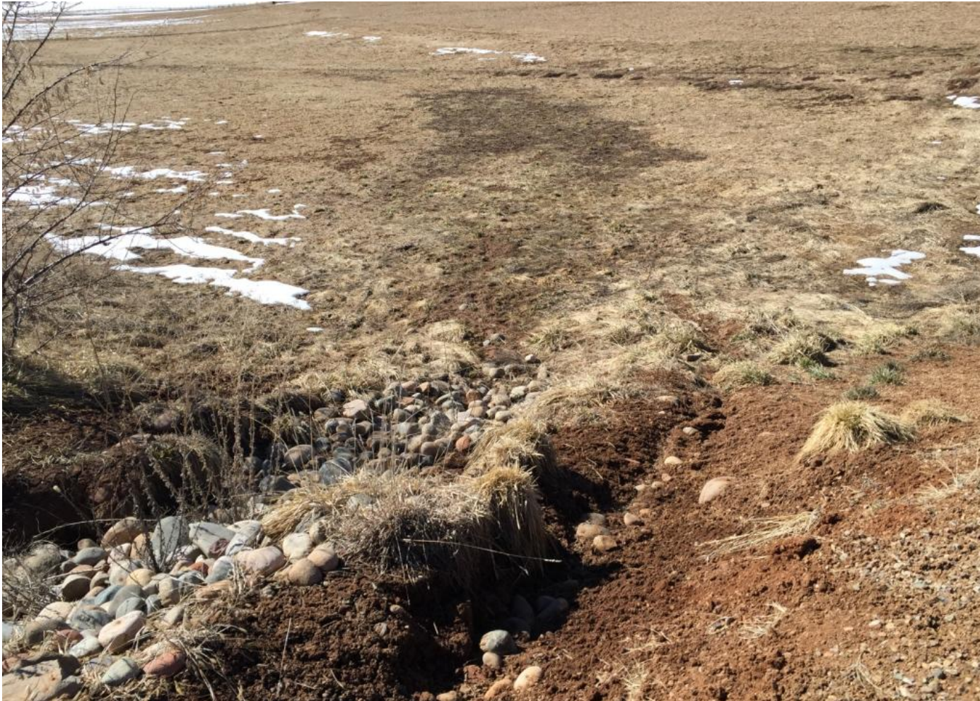
Photo 1. View of stormwater erosion occurring at the well pad entrance, south of the access road. It is unclear if cobble lined channel was recently stabilized or if it needs additional stabilization. The channel on the right does not appear stabilized and needs BMPs.
