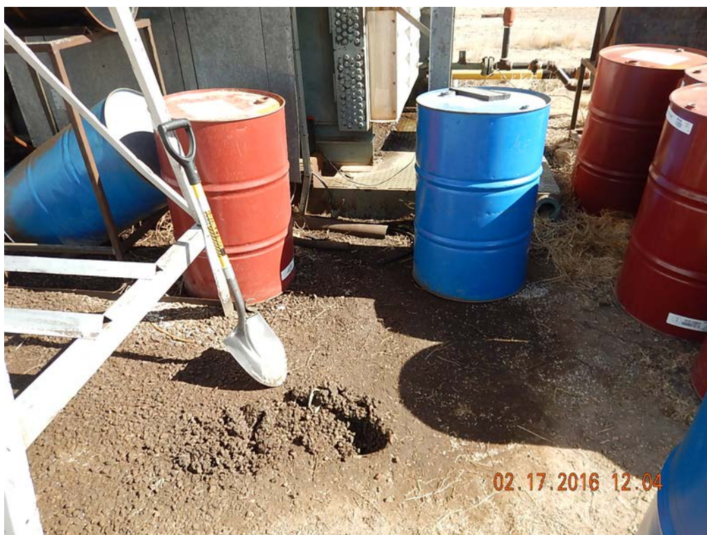
Figure 2 – Soil stained six to eight inches deep.
