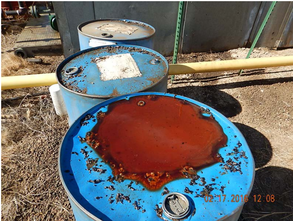
Figure 7 – Leaking barrels of motor oil stored on site.
