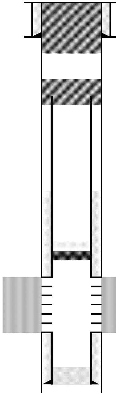
Cut surface casing off 6'-8' below surface.
