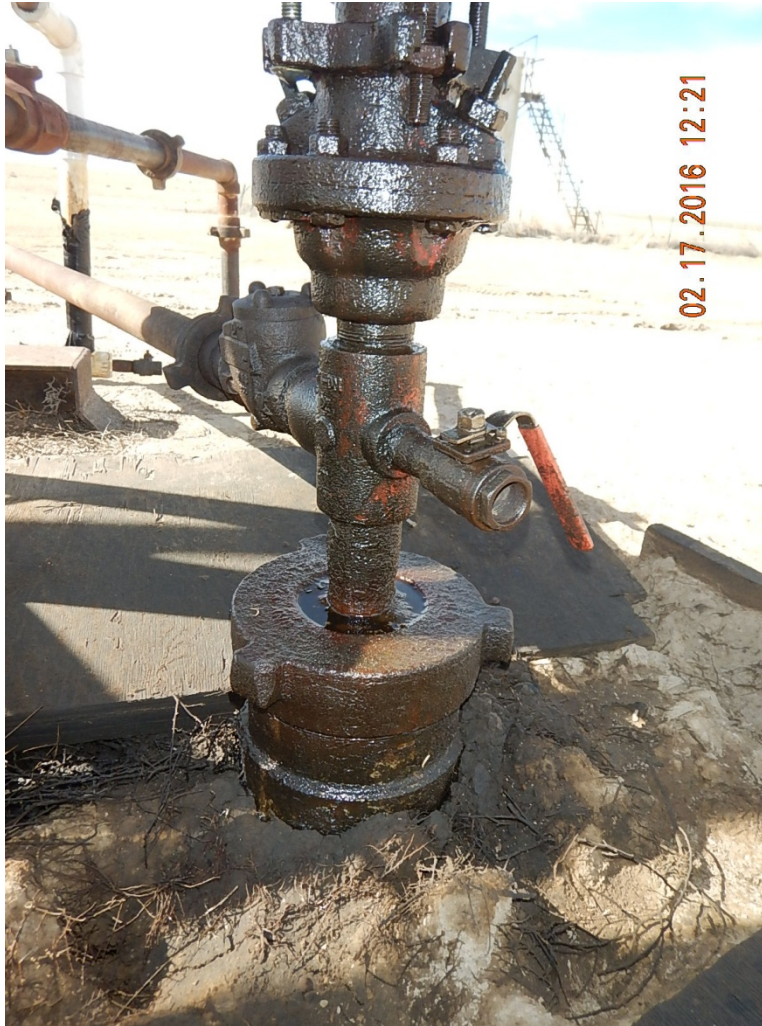
Figure 2 – Wellhead covered in oil and stained soil.
