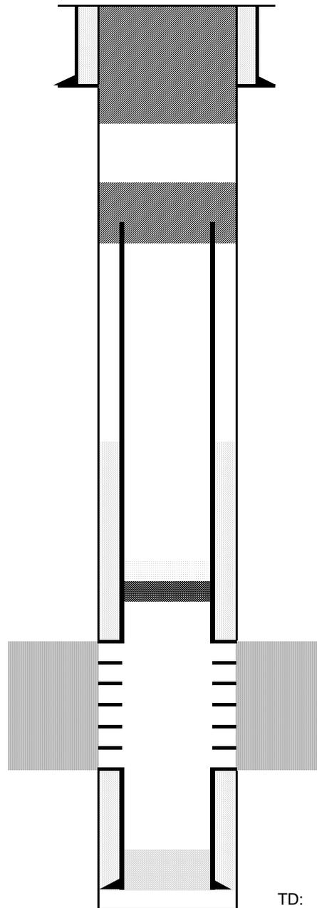
Cut surface casing off 6'-8' below surface.
