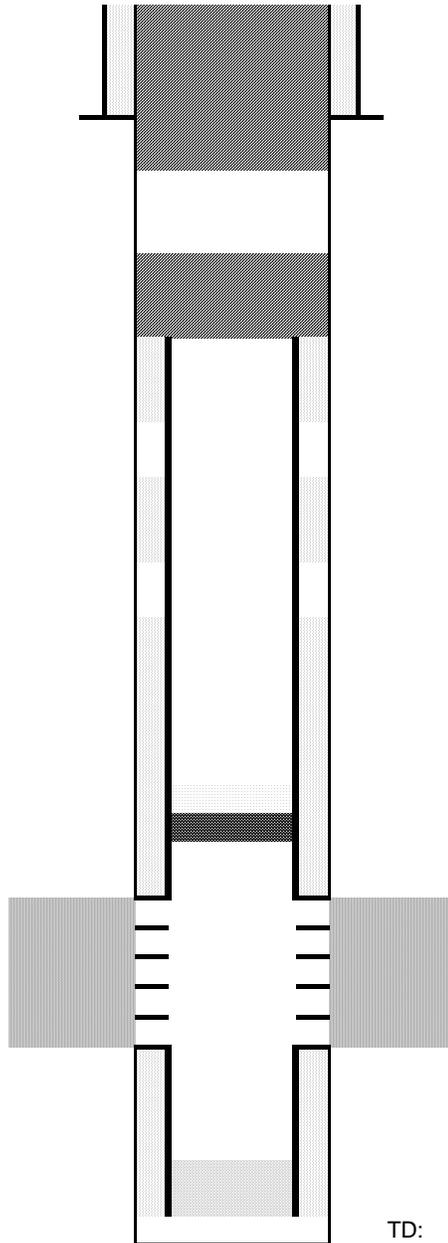
Cut surface casing off 6'-8' below surface.
