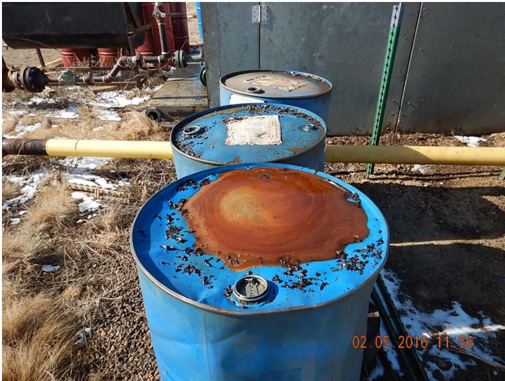
Figure 5 – Leaking barrels stored on location
