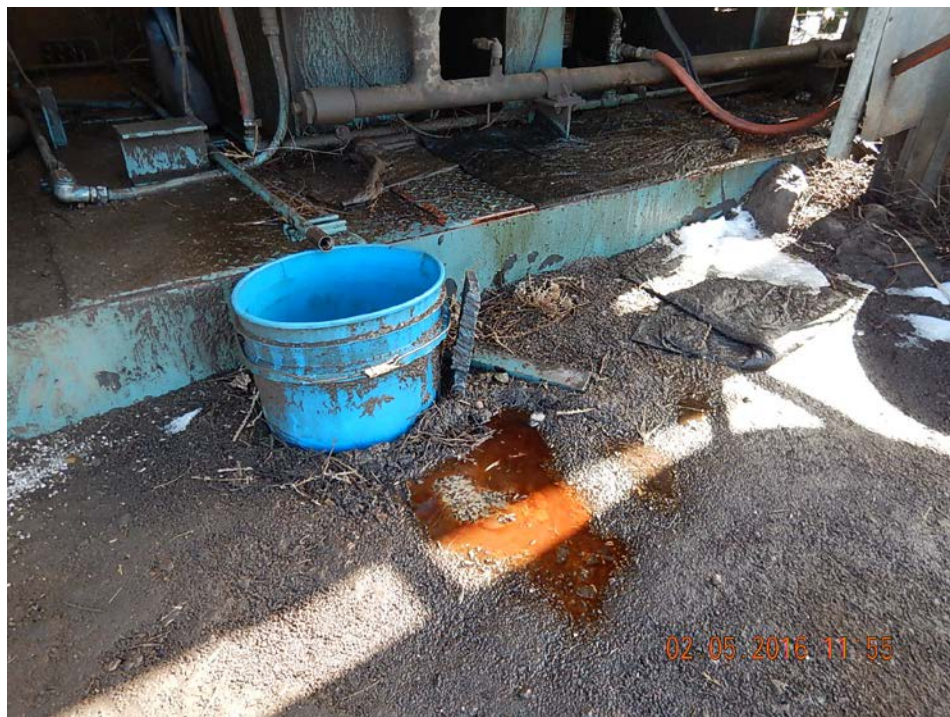
Figure 2 – Free product and stained soil on west side of compressor.
