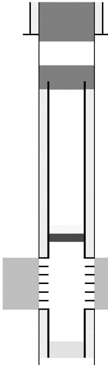
Cut surface casing off 6'-8' below surface.
