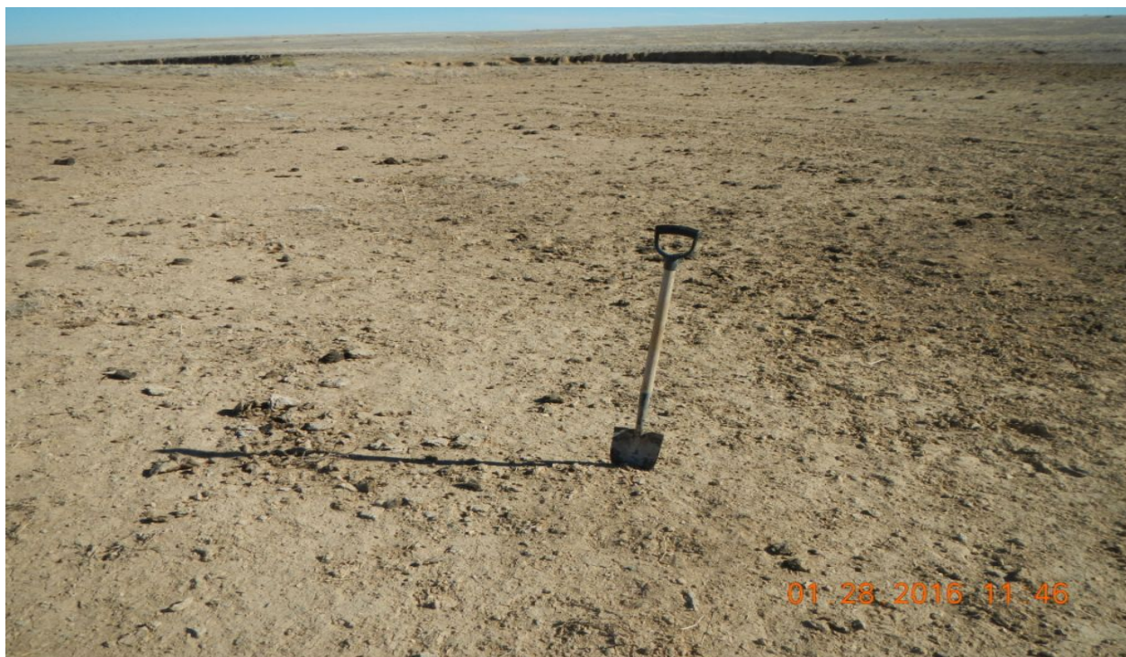
photo 9: Facing east at the location. Shovel was used to determine compaction. Soils were heavily compacted throughout the site.
