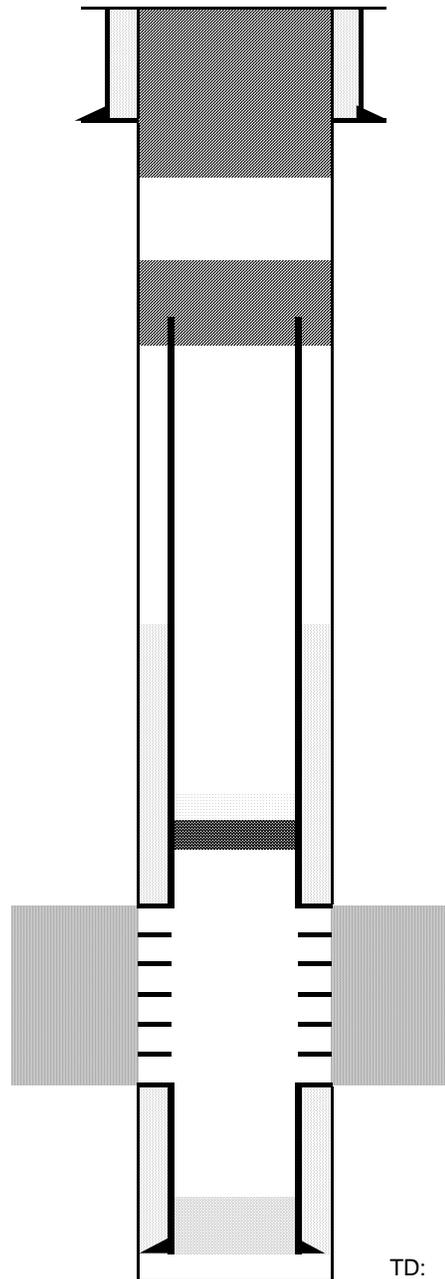
Cut surface casing off 6'-8' below surface.
