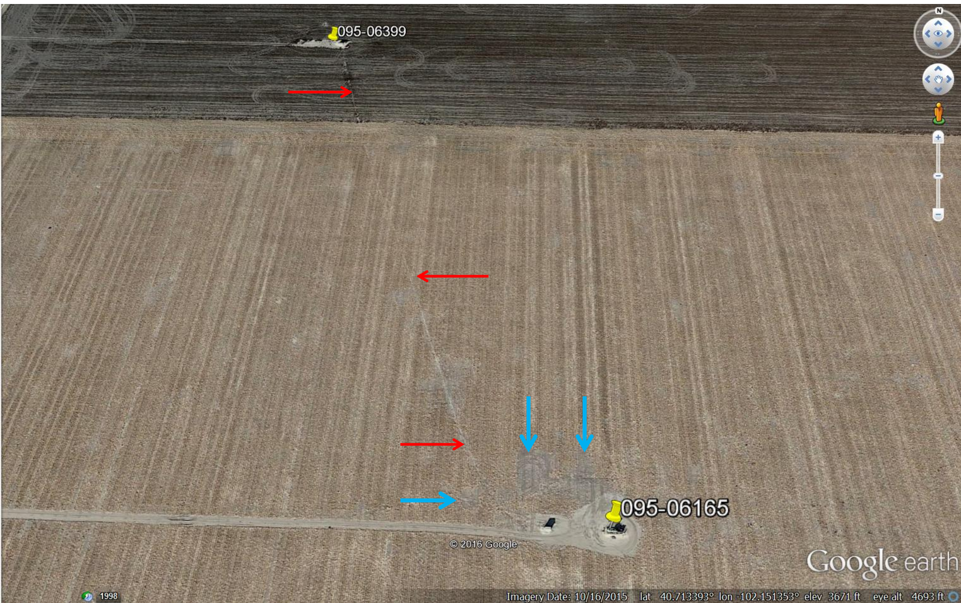
Figure 6: Aerial image of wells 095-06165 and 095-06399. Blue arrows indicates portions of interim area with sparse cover and bare soil. Red arrow indicates pipeline between wells with subsidence concerns.
