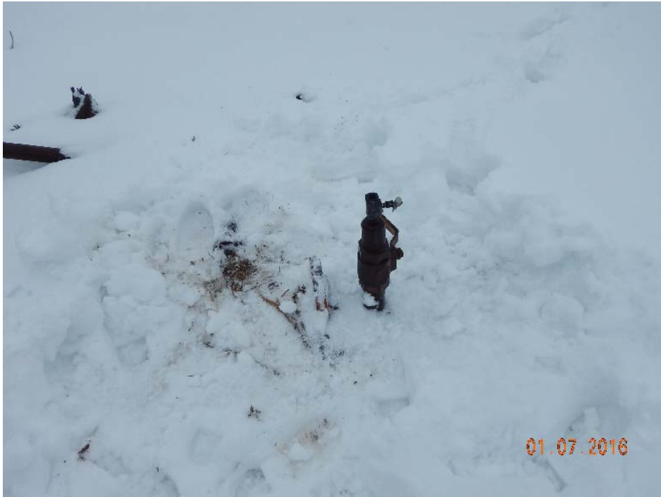
Wellhead Shut in, New Ball valve and Needle valve
