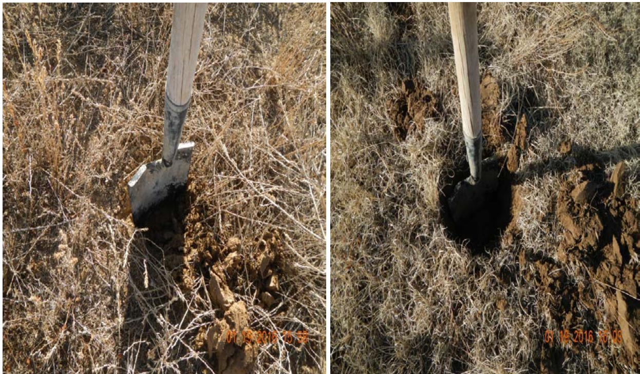
Photo 30: Soil compaction comparison indicated soils are more compacted at the disturbed location in comparison to the undisturbed soils. Photo on left is at location. Photo on the right is off location.
