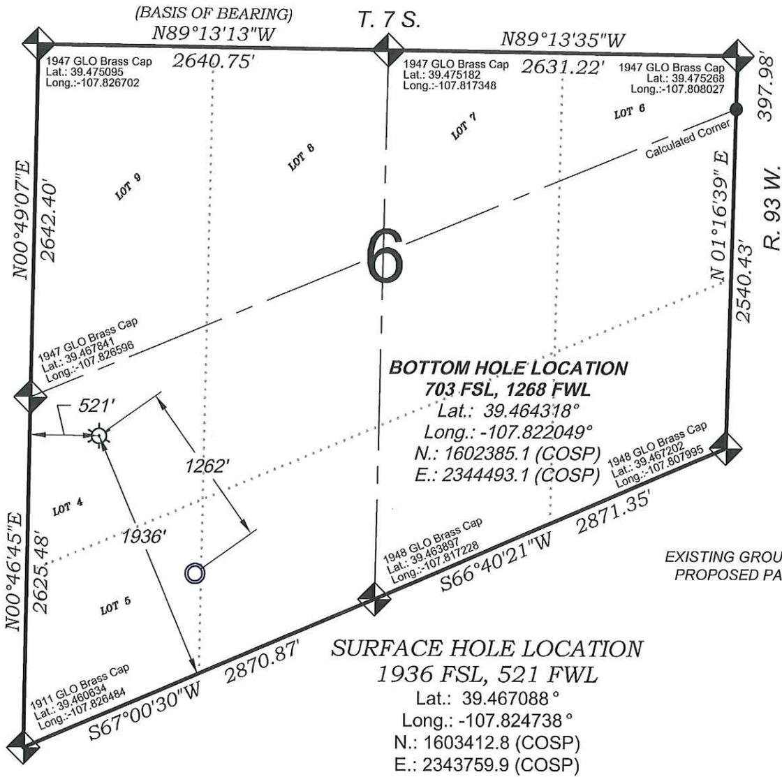
SEE CONSTRUCTION LAYOUT PLAT FOR VISIBLE IMPROVEMENTS WITHIN 500' OF THIS LOCATION
