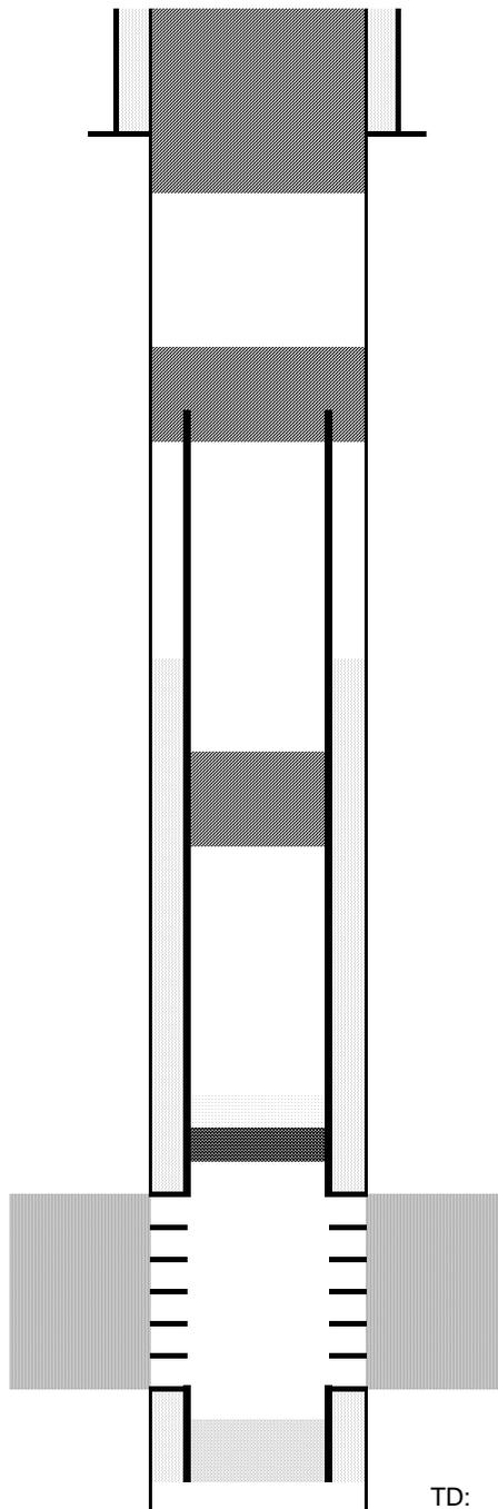
Cut surface casing off 6'-8' below surface.
