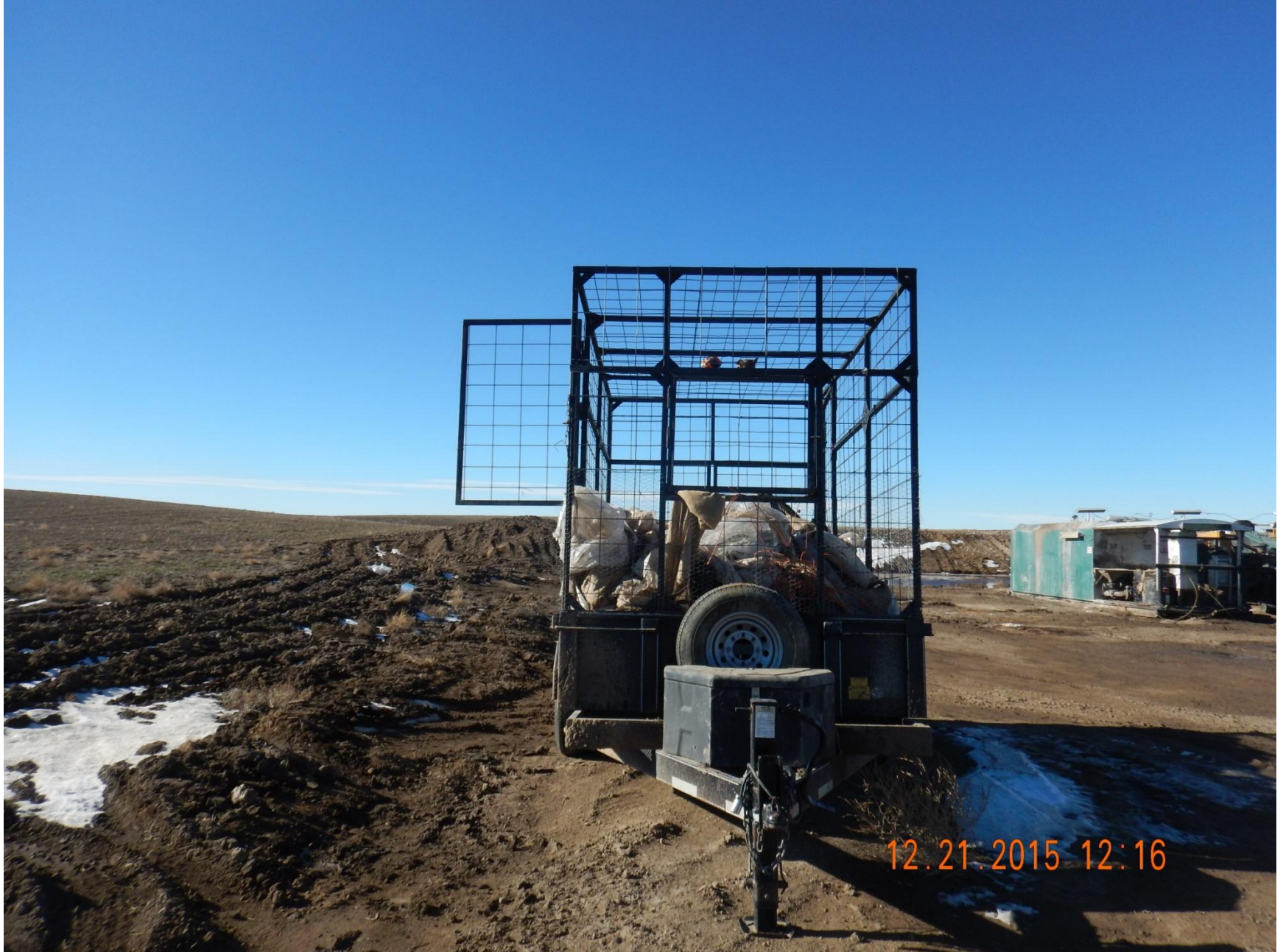
Figure 6: Photo taken from southeast end of location, facing west. Photo shows caged-trailer used for debris management. Note door to cage not properly shut.
