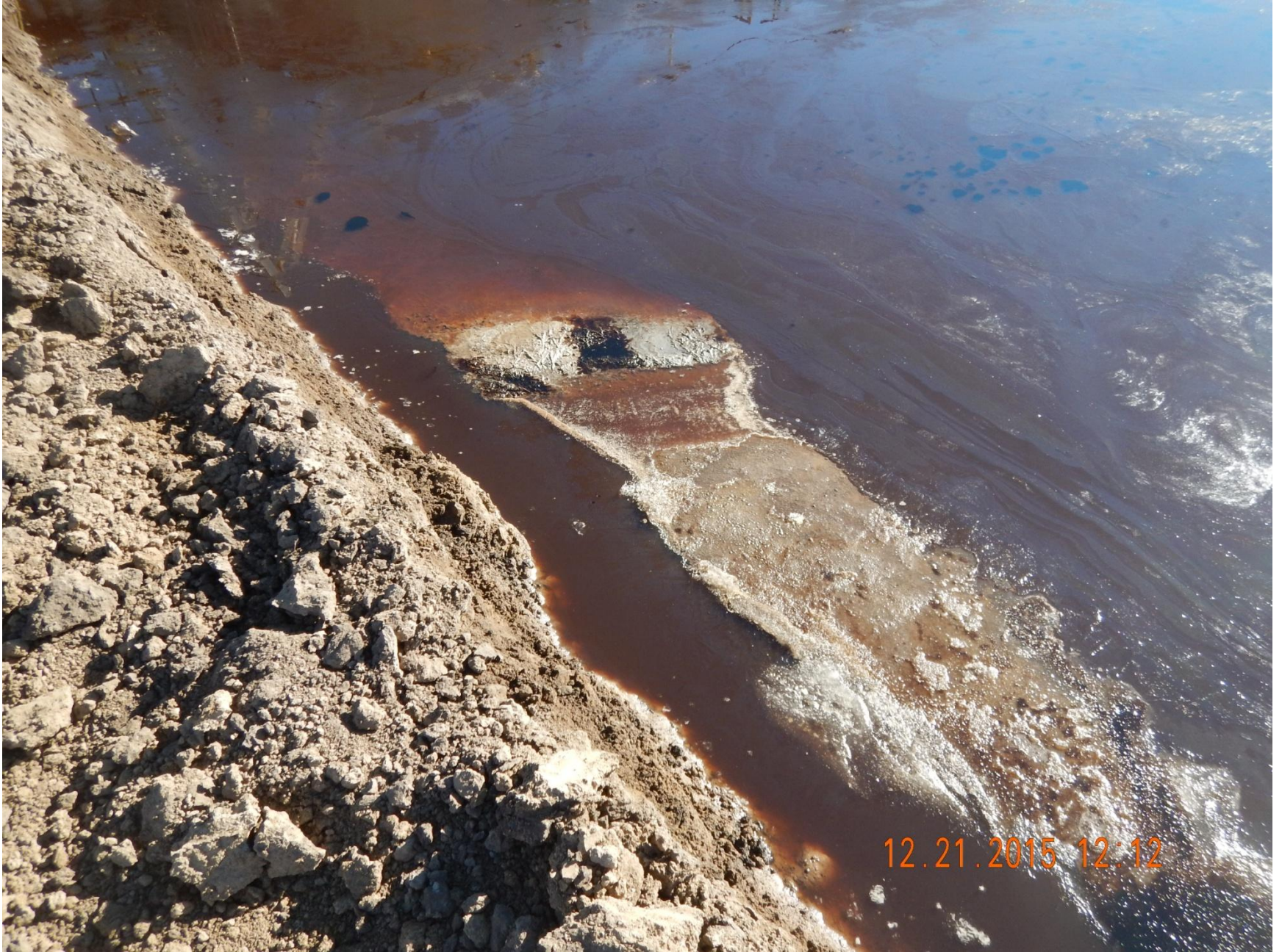
Figure 15: Photo taken at southern pit. Photo shows oily water. Pit does not appear to be lined.
