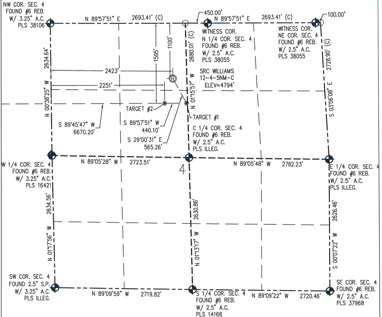
**N** IN ACCORDANCE WITH A REQUEST FROM CRAIG RASMUSON - SYNERGY RESOURCES, BASELINE ENGINEERING CORP. HAS DETERMINED THE LOCATION OF THE SRC WILLIAMS 12-4-5NM-C TO BE 1100' FNL AND 2423' FWL, AS MEASURED AT NINETY (90) DEGREES FROM THE SECTION LINE OF SECTION 4, TOWNSHIP 4 NORTH, RANGE 67 WEST AND THE BOTTOM HOLE LOCATION TO BE 1595' FNL AND 460' FWL OF SECTION 5, TOWNSHIP 4 NORTH, RANGE 67 WEST, 6TH PRINCIPAL MERIDIAN, WELD COUNTY, COLORADO.
