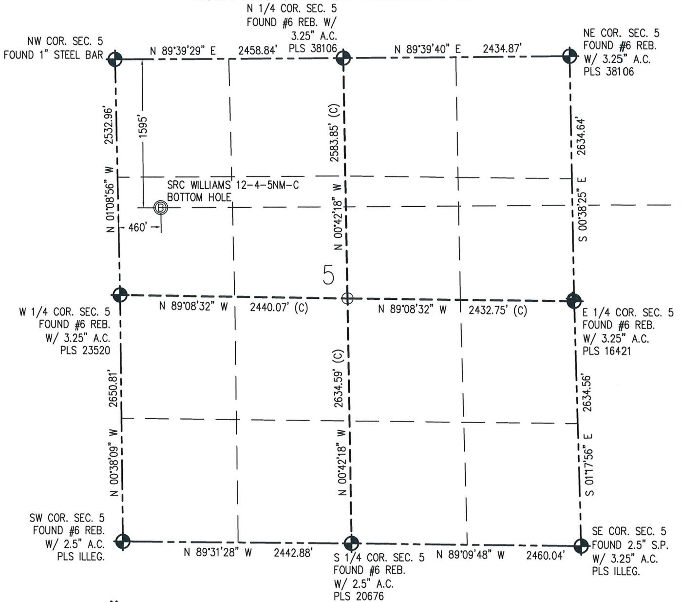
**N** IN ACCORDANCE WITH A REQUEST FROM CRAIG RASMUSON - SYNERGY RESOURCES, BASELINE ENGINEERING CORP. HAS DETERMINED THE LOCATION OF THE SRC WILLIAMS 12-4-5NM-C TO BE 1100' FNL AND 2423' FWL, AS MEASURED AT NINETY (90) DEGREES FROM THE SECTION LINE OF SECTION 4, TOWNSHIP 4 NORTH, RANGE 67 WEST AND THE BOTTOM HOLE LOCATION TO BE 1595' FNL AND 460' FWL OF SECTION 5, TOWNSHIP 4 NORTH, RANGE 67 WEST, 6TH PRINCIPAL MERIDIAN, WELD COUNTY, COLORADO.
