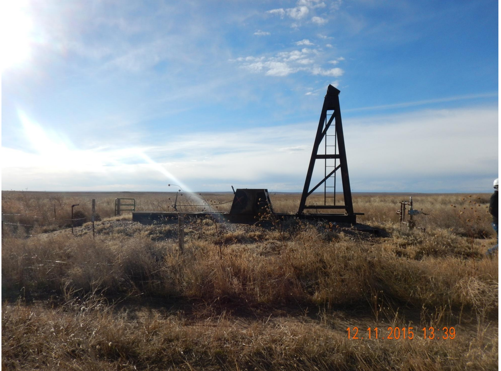
Figure 4: Photo taken from east end of location facing west. Photo shows dismantled pump jack. This is unserviceable equipment and needs to be removed.
