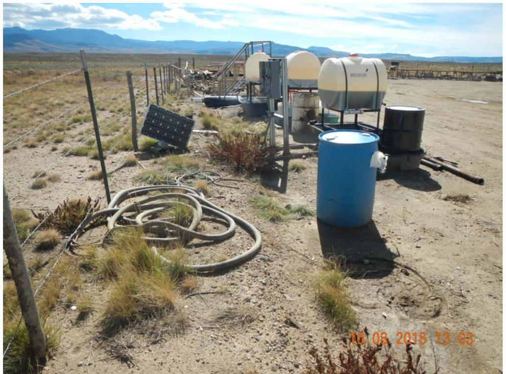
Close up of chemical storage with improper containment.
