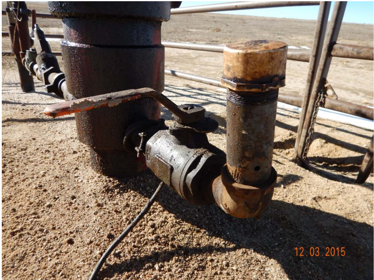
Figure 3 – Close up of vent nipple and closed valve.
