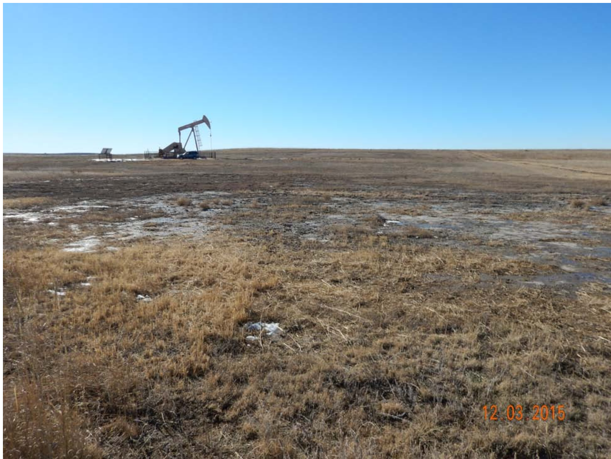
Figure 4 - View of bare soil, drilling fluid, and stressed vegetation northeast of well pad looking southwest.
