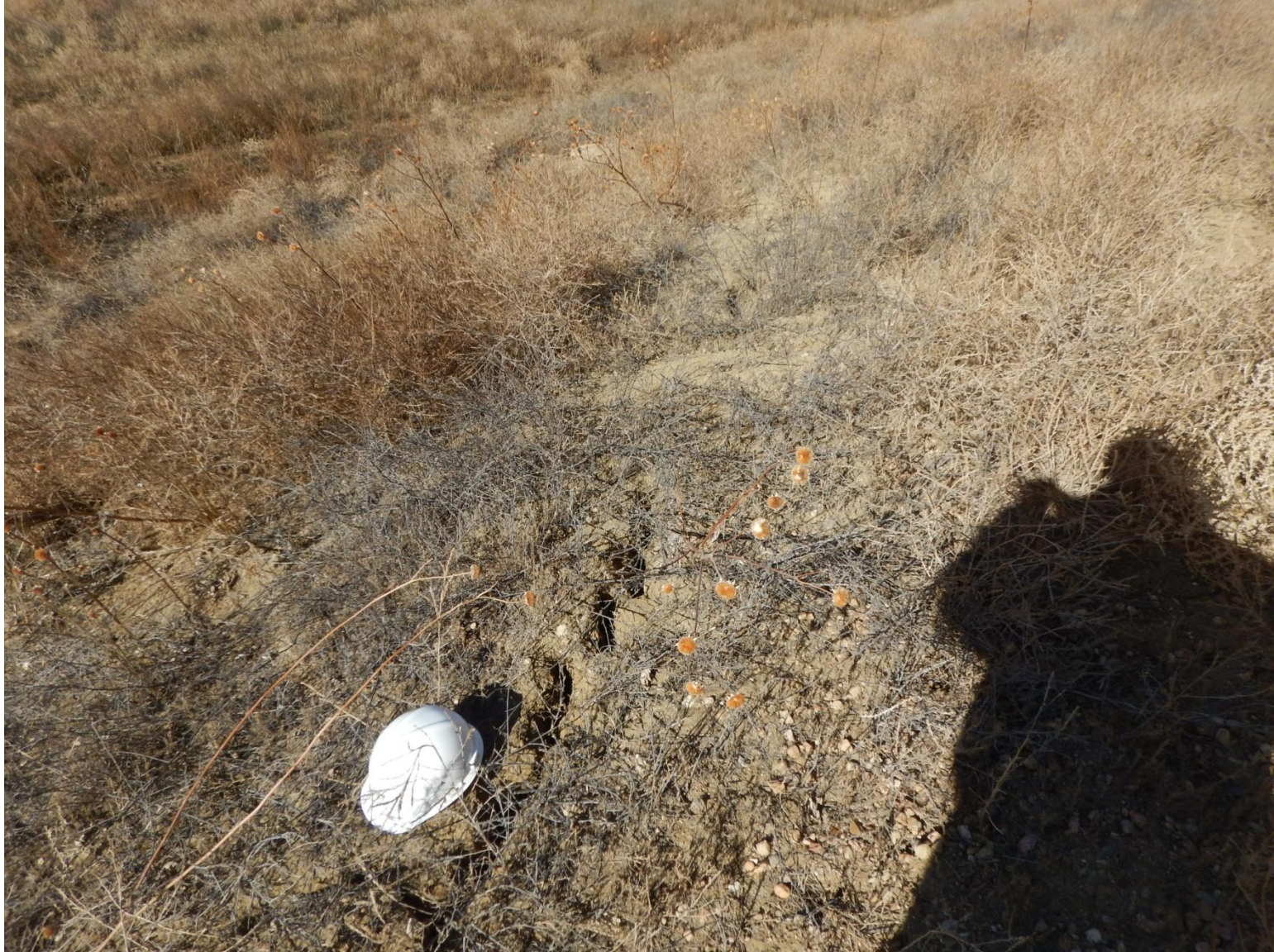
Photo 3: Photo taken from western side of location. Photo shows crack forming on slope, this is an indication of soil erosion occurring on slope.
