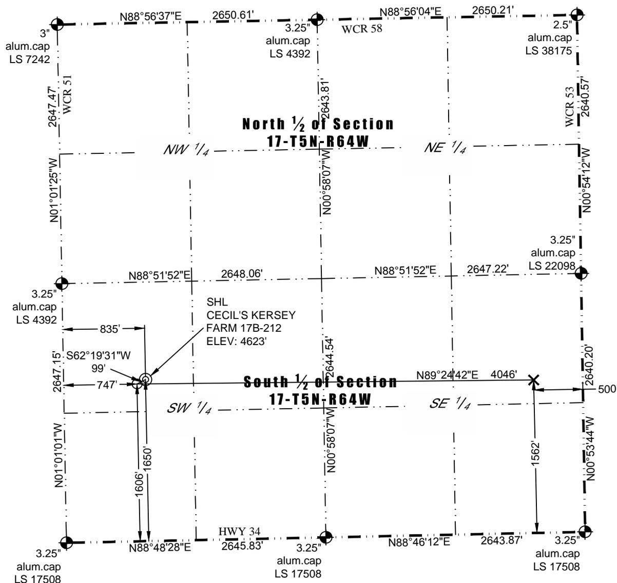
In accordance with a request from Barney Hammond of PDC Energy, Inc., Washburn Land Surveying, LLC has determined the location of the **CECIL'S KERSEY FARM 17B-212** well site to be SHL: 1650' FSL and 835' FWL, (BHL: 1562' FSL and 500' FEL), as measured at ninety (90) degrees from the section lines of Sections 17, Township 5 North, Range 64 West of the 6th Principal Meridian, Weld County Colorado.
