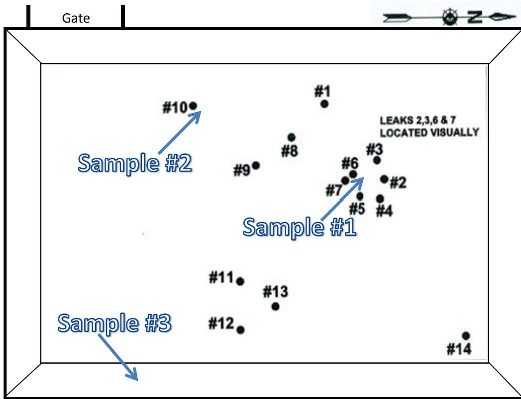
FIGURE 1 APPROXIMATE LOCATIONS OF LEAKS IN THE ROAN CREEK EVAPORATION POND
