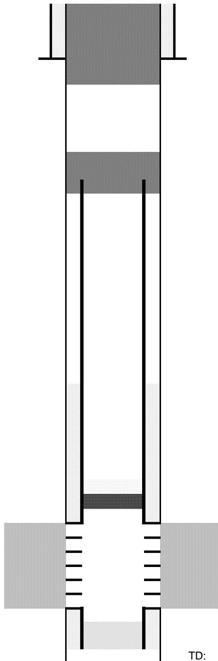
Cut surface casing off 6'-8' below surface.
