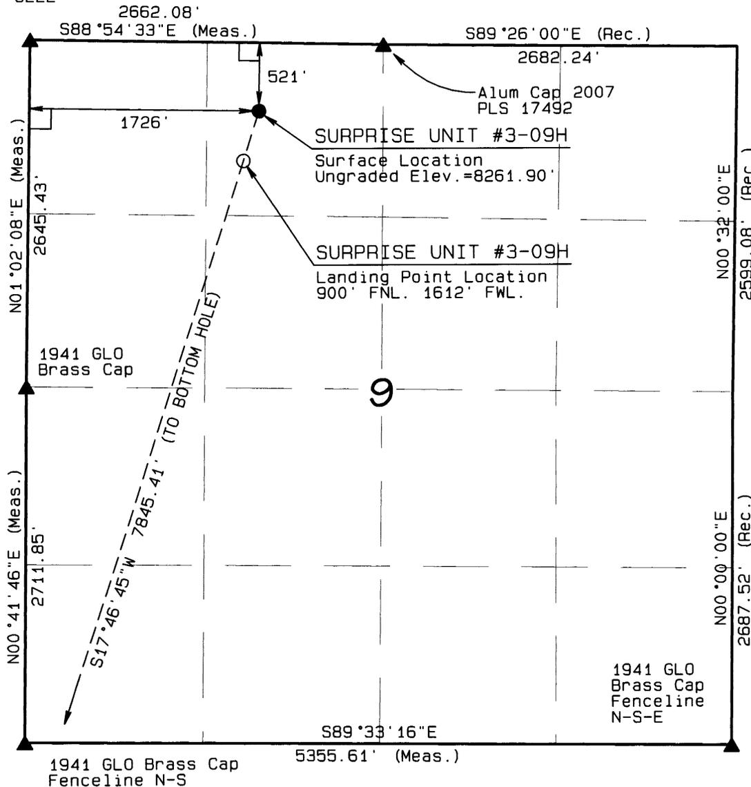
Surface Hole location, SURPRISE UNIT #3-09H as shown in the NE1/4NW1/4 of Section 9, T6N, R80W, 6th P.M., Jackson County, Colorado.
