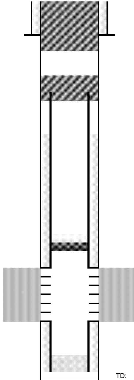
Cut surface casing off 6'-8' below surface.
