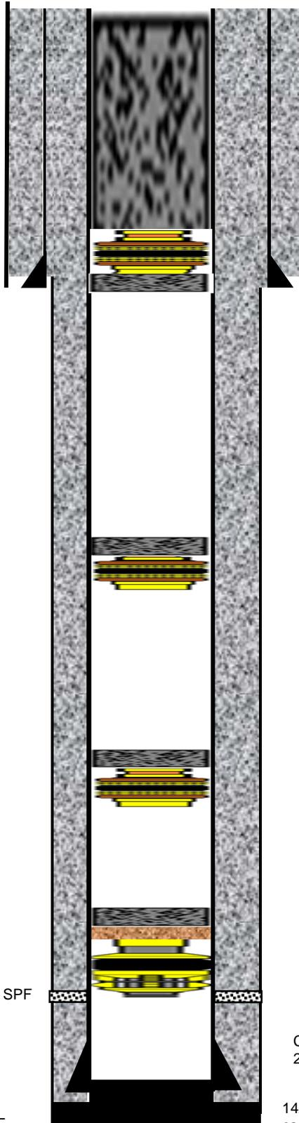
Hole filled from 100" to surface with cement
