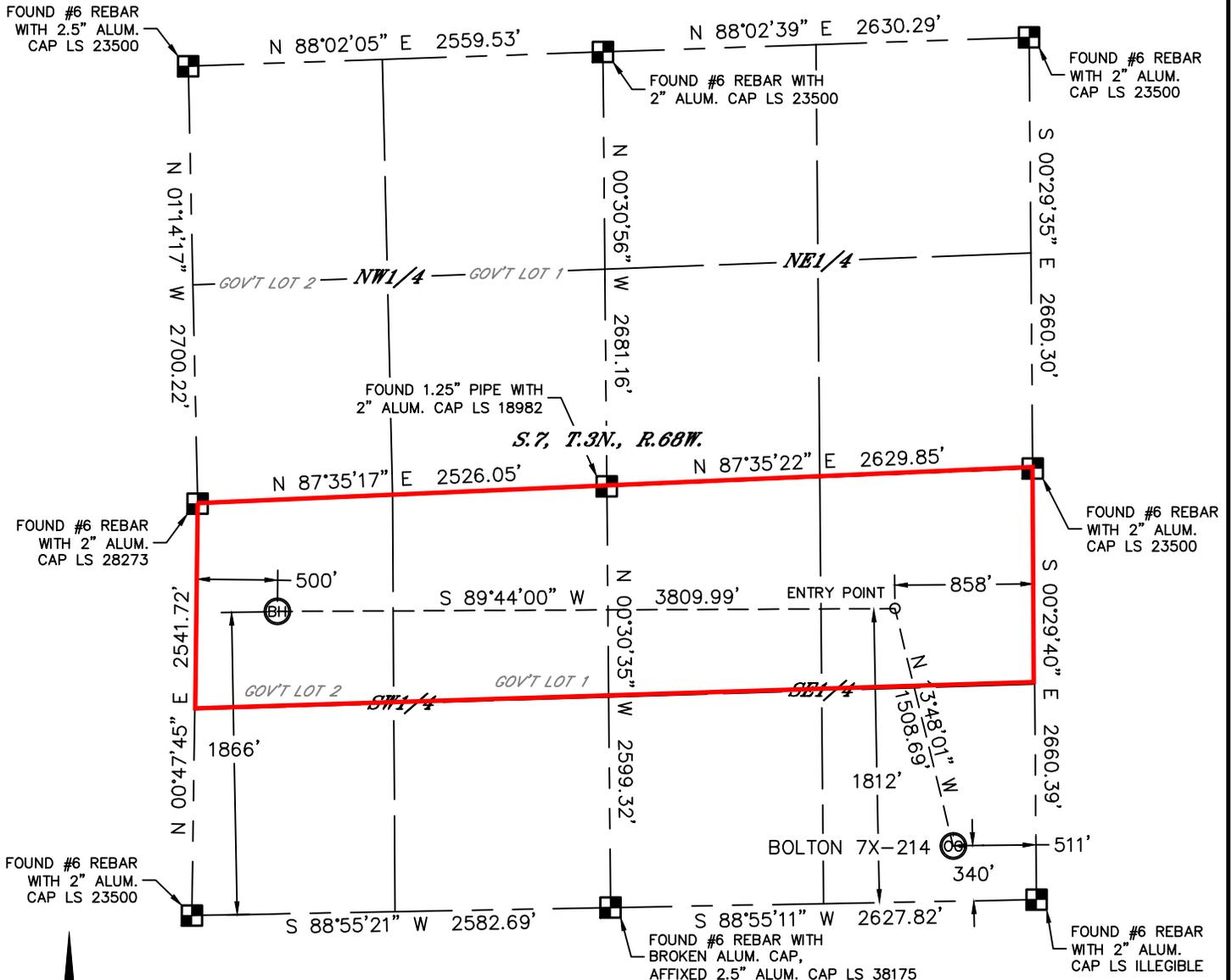
In accordance with a request from Jake Bragg with PDC ENERGY Lat40°, Inc. has determined the surface location of the BOLTON 7X-214 to be 340' from the SOUTH line and 511' from the EAST line and the bottom hole to be 1866' from the SOUTH line and 500' from the WEST line as measured at right angles from the section lines of Section 7, Township 3 North, Range 68 West of the Sixth Principal Meridian, County of Weld, State of Colorado.
