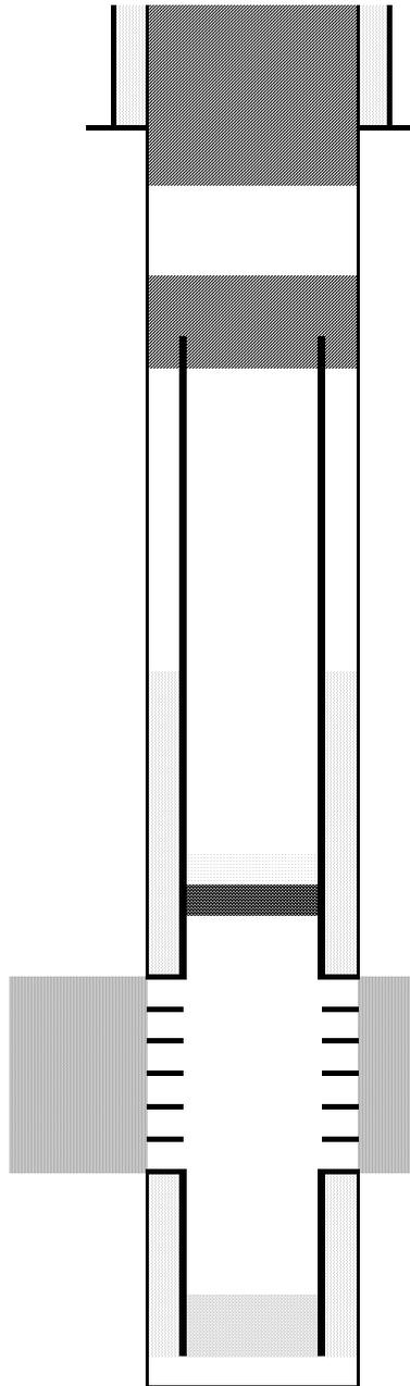
Cut surface casing off 6'-8' below surface.
