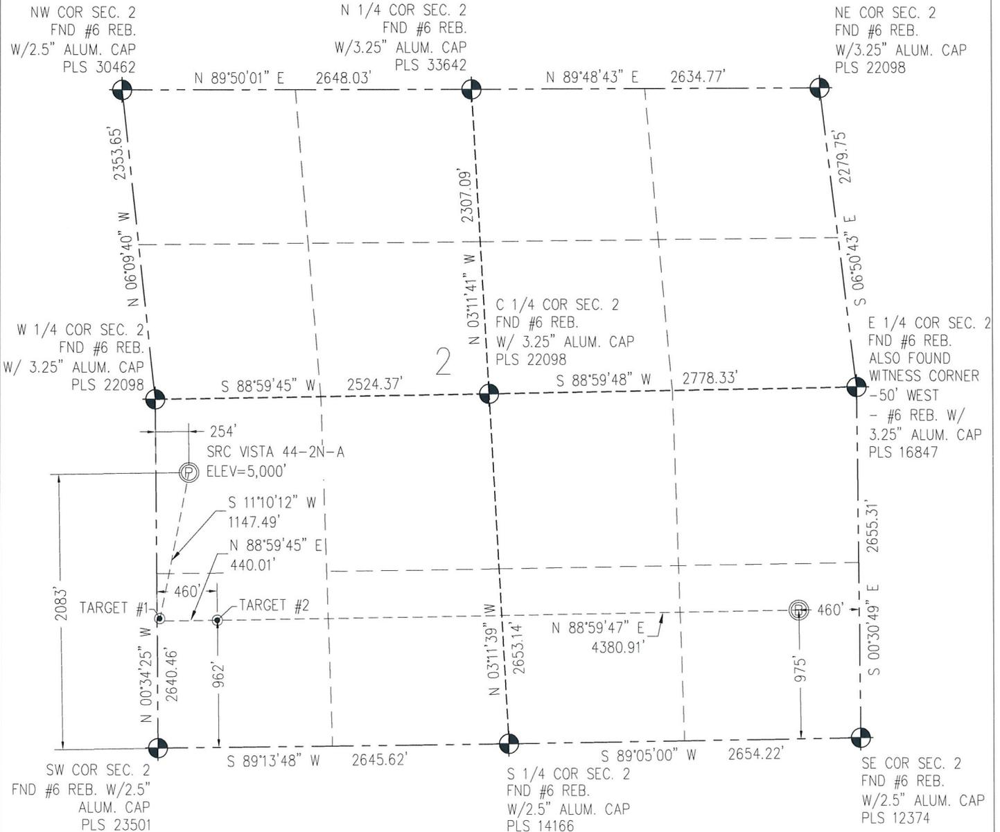
**N** IN ACCORDANCE WITH A REQUEST FROM CRAIG RASMUSON - SYNERGY RESOURCES, BASELINE ENGINEERING CORP. HAS DETERMINED THE LOCATION OF THE SRC VISTA 44-2N-A TO BE 2083' FSL AND 254' FWL, AS MEASURED AT NINETY (90) DEGREES FROM THE SECTION LINE OF SECTION 2, TOWNSHIP 4 NORTH, RANGE 68 WEST AND THE BOTTOM HOLE LOCATION TO BE 975' FSL AND 460' FEL OF SECTION 2, TOWNSHIP 4 NORTH, RANGE 68 WEST, 6TH PRINCIPAL MERIDIAN, WELD COUNTY, COLORADO.
